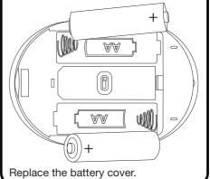
Only AA batteries of the type specified can be used. Do not mix old and new batteries.
